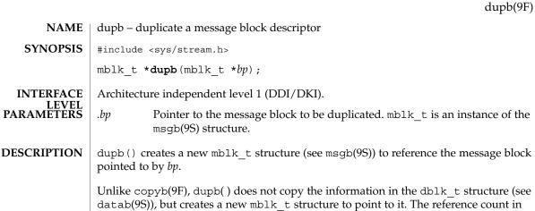
datab(9S)), but creates a new mblk\_t structure to point to it. The reference count in the dblk\_t structure (db\_ref) is incremented. The new mblk\_t structure contains the same information as the original. Note that b\_rptr and b\_wptr are copied from the *bp*.
