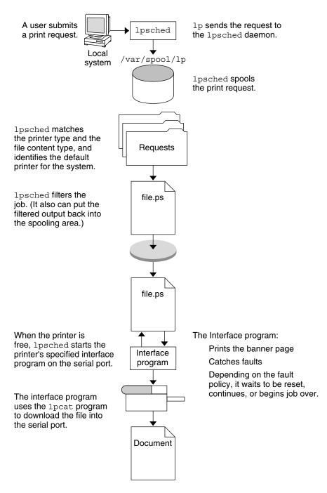
FIGURE 8–2 The Local Printing Process
