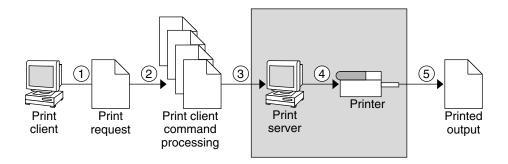
FIGURE 2-4 The Print Server Sends a Print Request to the Printer
