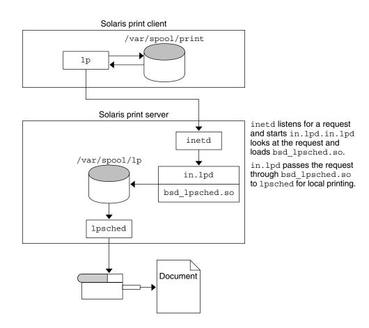
FIGURE 8–5 Printing Between a Solaris Print Client and a Solaris Print Server
