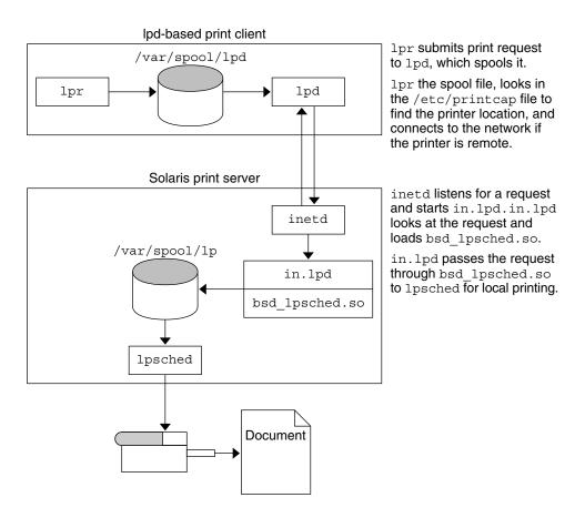
FIGURE 8-4 Printing Between a 1pd-based Print Client and a Solaris Print Server
