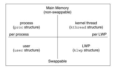
FIGURE 22-1 Process Structures
