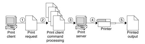
FIGURE 2-1 Overview of the Print Client Process
