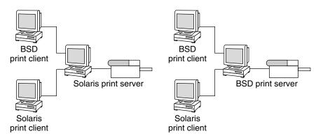
FIGURE 3-2 Solaris and lpd-Based Systems Print Configuration
