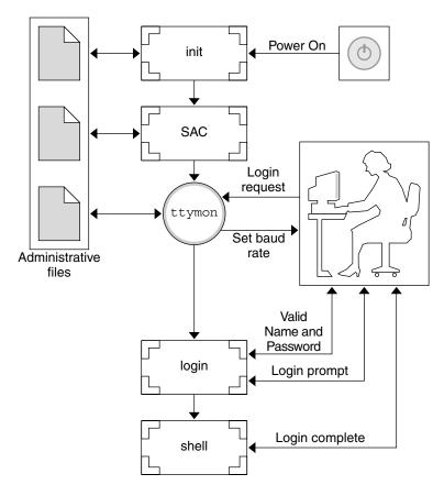
FIGURE 12-1 How ttymon Helps Process a Login Request
