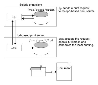
FIGURE 8-3 Printing Between a Solaris Print Client and a 1pd-based Print Server
