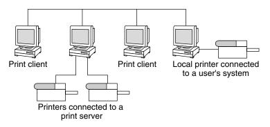
FIGURE 3-1 How to Distribute Printers on a Network
