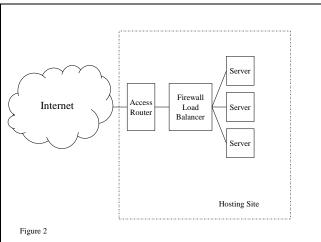
The typical scenario for hosting services is shown in Figure 2. The SLAs offered by hosting providers deal with the uptime and performance of the servers that are being hosted. These operators are only able to control the server side of the total
