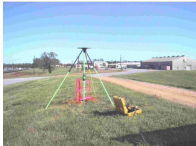
Figure 6-1. Control survey observing scheme on Mississippi River and control point baseline occupation at Memphis District Ensley Boatyard (Memphis District and 3001, Inc.)
