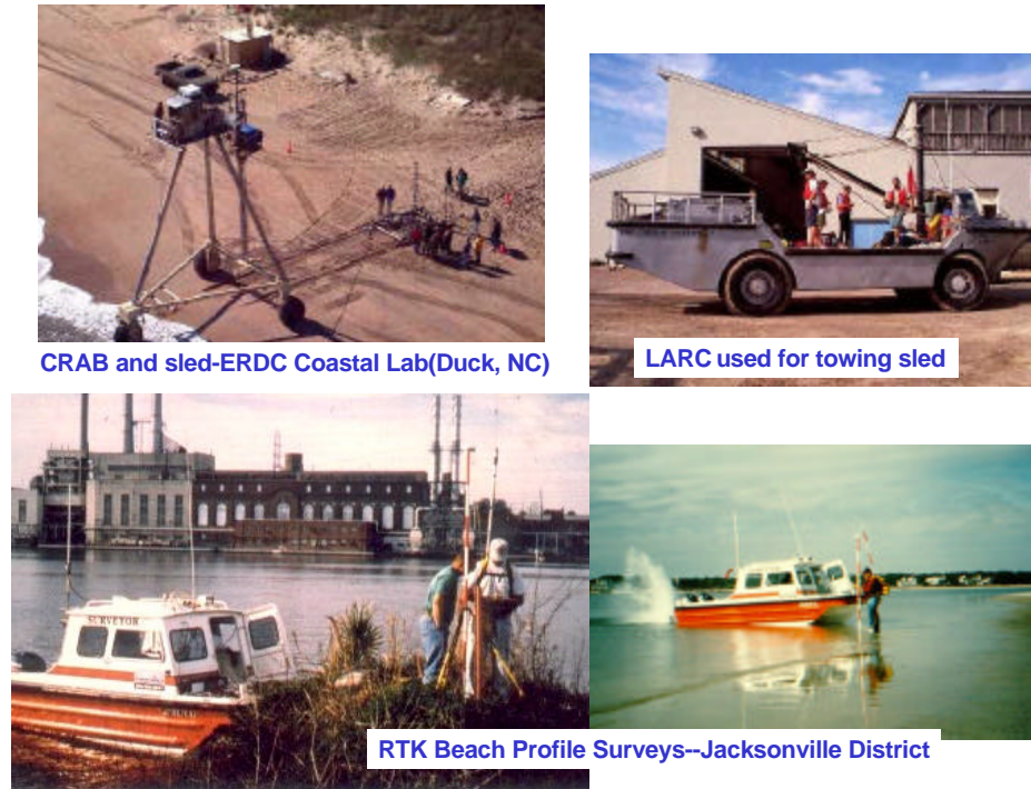
Figure 6-12. Differential GPS controlled beach survey platforms--for coastal engineering surveys (ERDC/Coastal & Hydraulics Lab, Jacksonville District, Arc Surveying & Mapping, Inc.)
