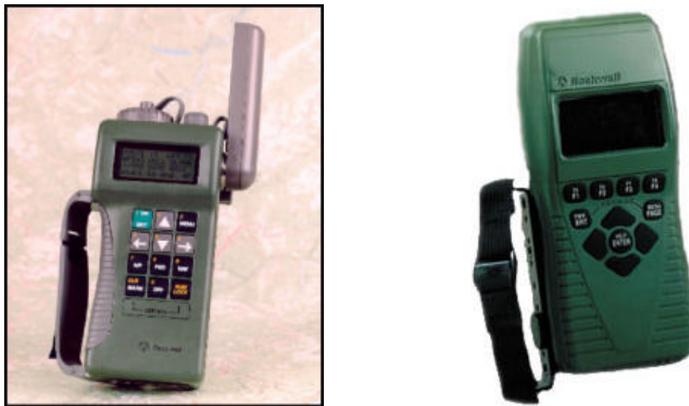
Figure 7-2. PLGR+96 (left) and PLGR II (right)
