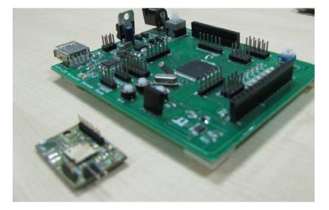
Snapshot of Wi-Fi based Wireless Sensor Network development platform
