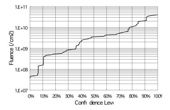
Figure A.3 — Example of Confidence Level of 4-8MeV Proton for 1-year duration
