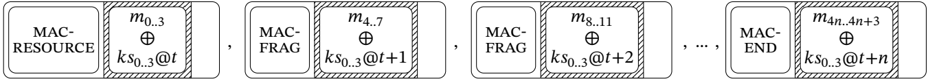
Figure 12: Single message m divided over n + 1 four-bit fragments. m_{i..j} denotes bits i to j of m .
