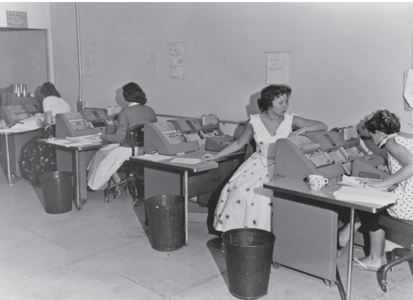
Keypunch operators created duplicate stacks of punched cards for each program, comparing them to ensure accuracy.
