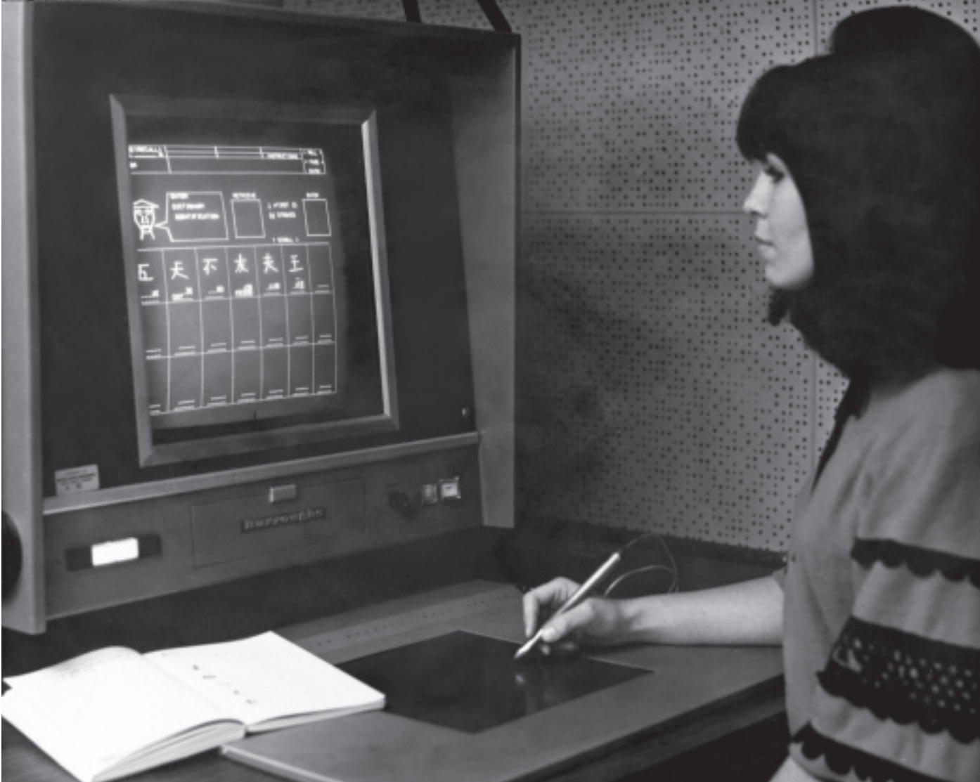
The RAND tablet and the videographic system could be used to look up handwritten ideographs in an electronic Chinese dictionary.
