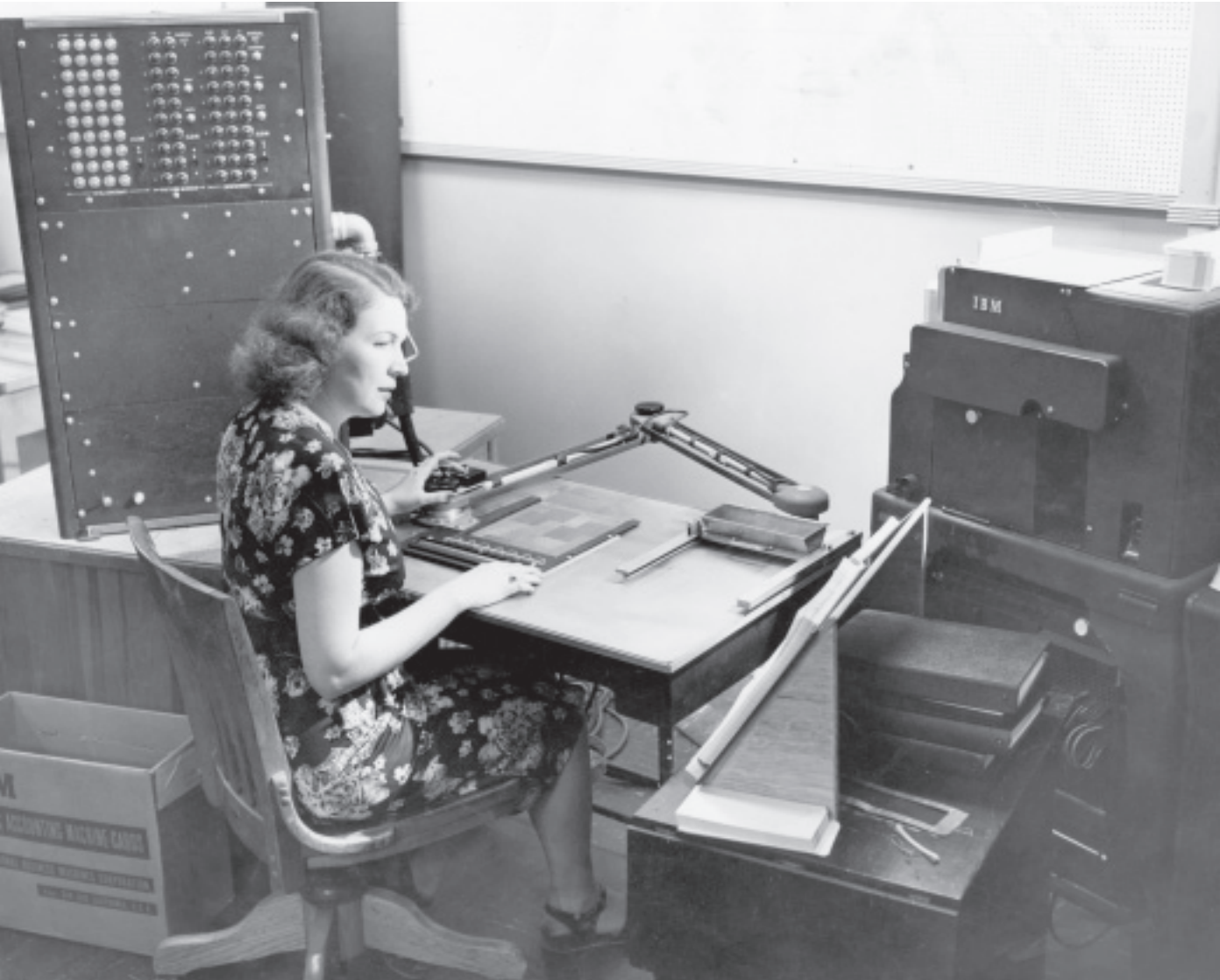
RAND built a physical analog computer called the coverage machine that dropped thousands of ball bearings (targets) on bomb-pattern plates.
