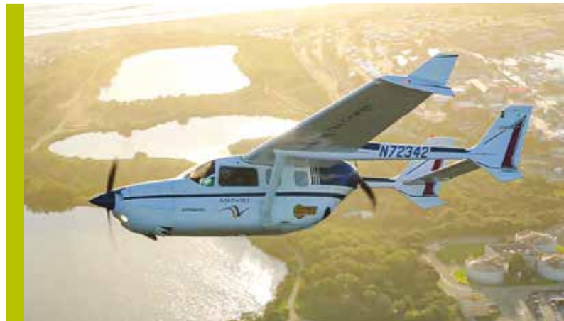
Above: The Ampaire Electric EEL is a Cessna 337 Skymaster with an electric rear motor. Ampaire.
